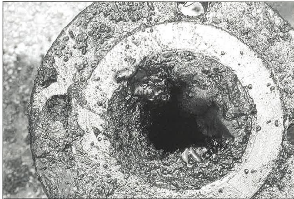
Before - this oil line has very little flow capacity
